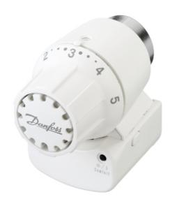
control up to four energy saving times per day can be preset in the thermostat. In case the wireless control is not active the RA plus-w will switch the modes independently. The energy saving times can always be changed and manually overwritten by pressing the button on the device. The two AA batteries last for up to four years. The unit will send a warning via wireless connection and give a local LED warning when batteries need to be replaced.
