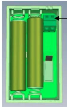
Terminal blocks for external wiring
