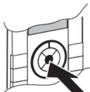
A confirmation window appears. Programming status/learning mode is activated for about 5 seconds. During this time, the radio central unit is detected by the radio USB data interface and integrated into the project in the CONNECT radio configurator.
