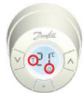
If no connection can be made, the alarm and antenna symbols flash together.
