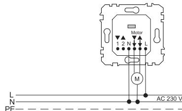
**Caution!** Phase potential is used for wiring and controlling several inserts. Therefore, use commercially available NYM cables for wiring.
