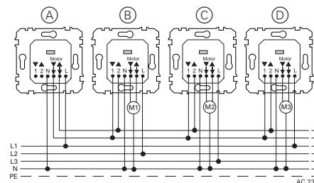
Inserts in central control spread over several phases. The inserts can be clamped onto different phases as required.
