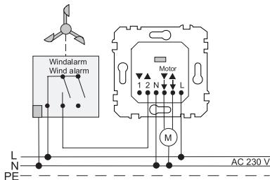
When the wind alarm is activated, the blinds are raised and remain locked in that position until the wind dies down. Therefore, the blinds cannot be operated manually or automatically.
