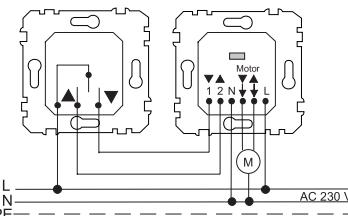
When the push-button of the roller shutter rocker button is briefly operated, the blind control insert does not switch to self-locking (continuous operation). You can also bring the blinds into the required position by holding the rocker button down. Recommendation: To wire two inserts between the inserts, use a cable of 5 x 1.5 mm<sup>2</sup> (1, 2, L, N, PE).
