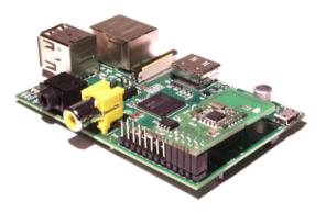
Gateway. If implements the Z-Wave transceiver including the low level network protocol, the Z-Wave application level protocol and a Java Script based automation engine.
