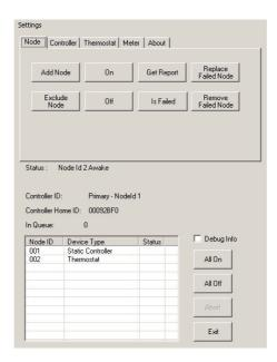
All other switching functions of the Node-Tab are designed for the administration of the network and not needed for RA plus-w thermostats. Once all thermostats are included successfully switch over to the Thermostat-Tab.
